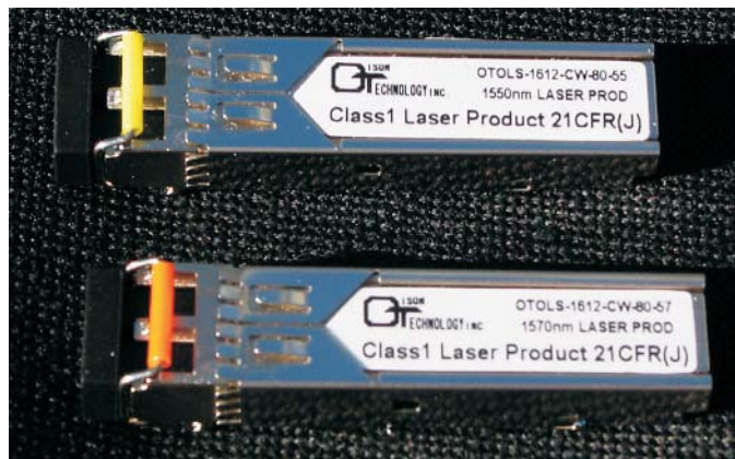
Figure 3 - Single-mode CWDM SFP Modules with Dual LC Connectors
