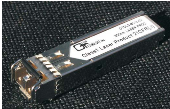
Figure 2 - Multimode 850nm SFP Module with Dual LC Connectors
