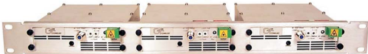
Three (3) OTLT-87XX-40-SA Transmitters on an Optional OTLL-RMKIT-1
